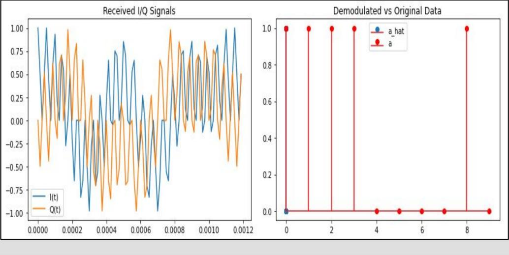
The GMSK demodulated signal is the same as the original input signal.
