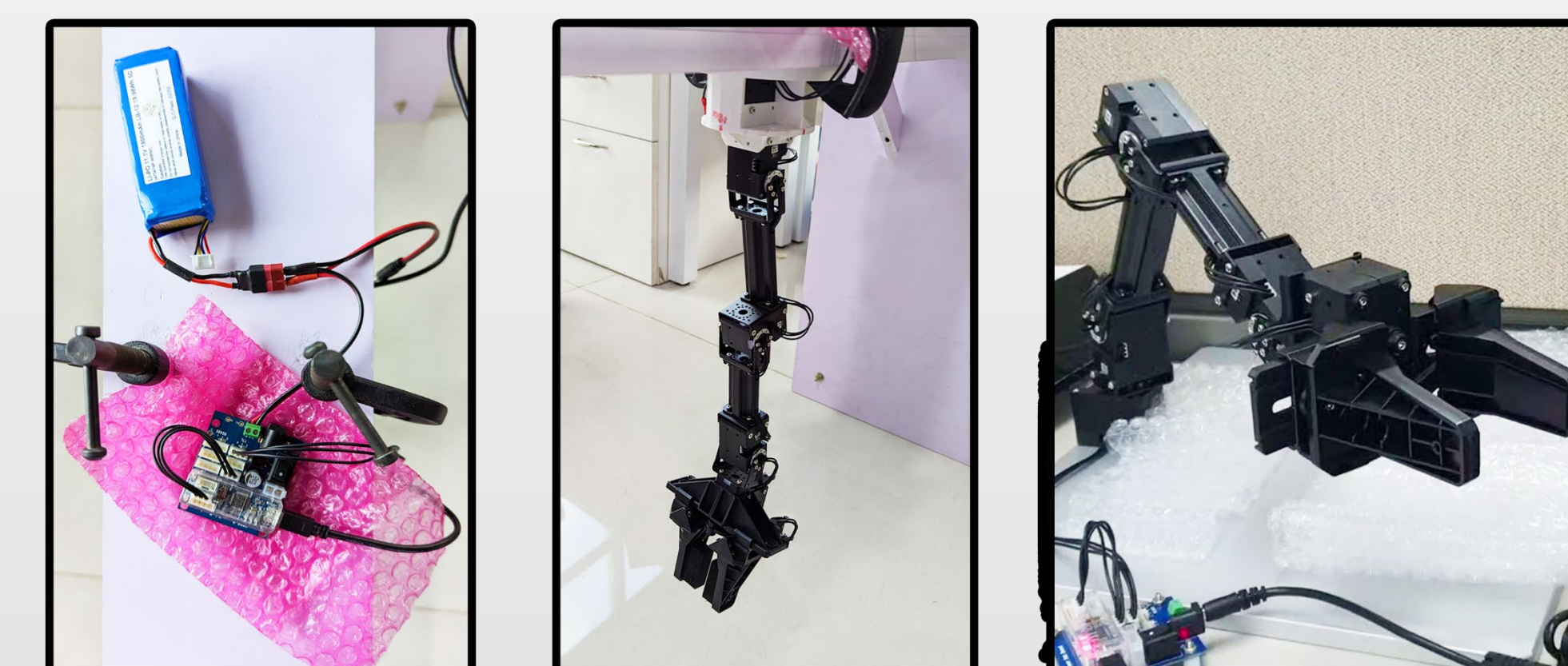
Figures above shows the assembled hardware kit of OpenManipulatorX interfaced to the Laptop using U2D2.
